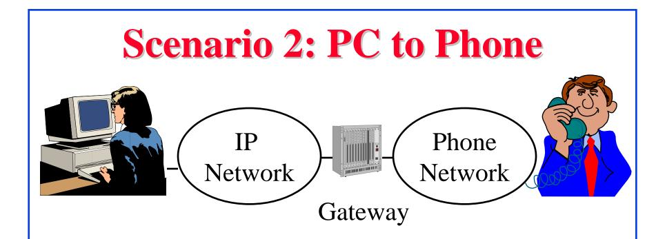
Need a gateway that connects IP network to phone network (Router to PBX)
