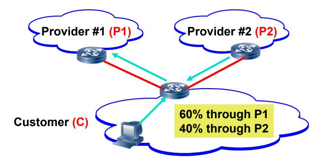
Solution: Border routers over-write source addresses in the outgoing packets. TE-proxy switches flows not packets.
