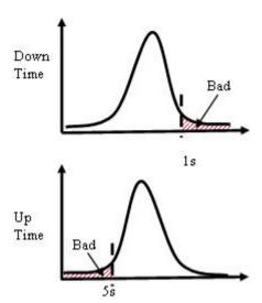
Fig. 5. Percentiles of downtime and uptime are better metric for sense and avoid applications than availability
