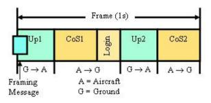
Fig. 3. L-DACS2 Physical Layer Framing
