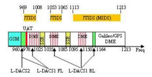
Fig. 4. L-band spectrum usage
