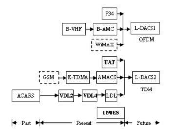
Fig. 1. Evolution of aeronautical datalinks
