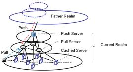
Fig. 6. Hybrid push/pull/caching mapping delivery
