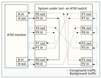
Figure 5. A scalable test configuration for measurement of MIMO latency using only two generator/analyzer pairs with 8port switch and a 7-to-7 straight connection configuration for the background traffic.
