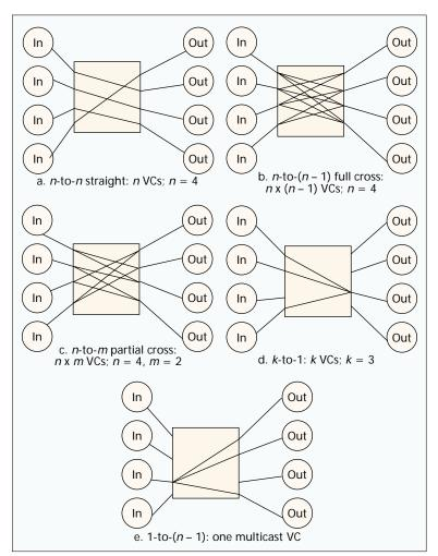
Figure 2. Connection configurations for throughput measurements.
