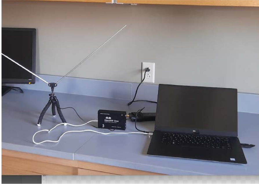
Figure 2: Transmitter Setup. From left to right: Dipole antenna, hackrf one SDR, Laptop running live image of pentoo linux executing the GNU radio flowgraph.
