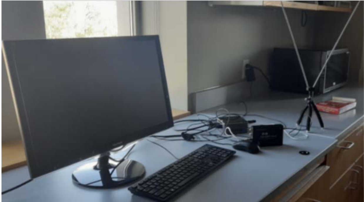
Figure 3: receiver Setup, from left to right: Desktop PC running live image of pentoo linux executing the receive GNU radio flowgraph, hackrf one SDR, Dipole antenna.
