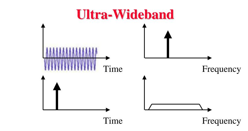
■ An impulse in time domain results in a ultra wide spectrum in frequency domain and essentially looks like a white noise to other devices
