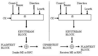
Fig 4. Air Interface Confidentiality Mechanism
