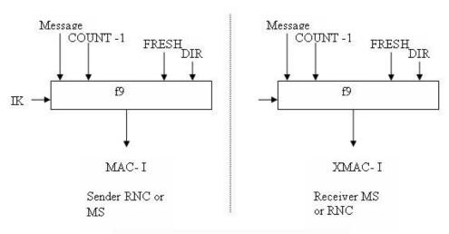
Fig 3. Signaling Data Integrity Mechanism
