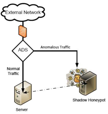
Figure 2. Segmenting traffic in a shadow honeypot system
