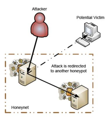
Figure 1. Redirecting an outbound attack in a honeynet
