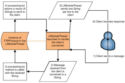
Figure 8. The FTP protocol's communication with a client through the processInput() method
