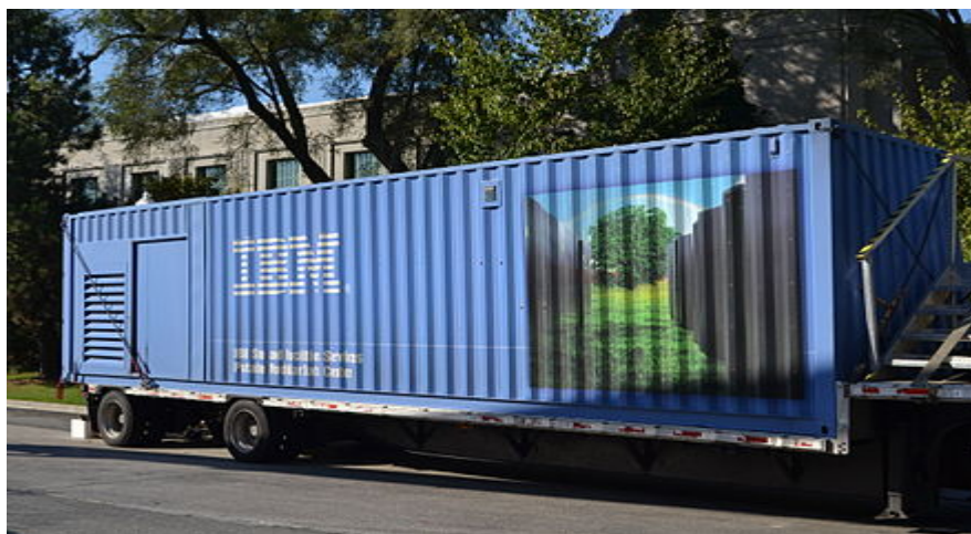
Fig. 2: A trailered modular data center by IBM[ wikipedia23 ]
