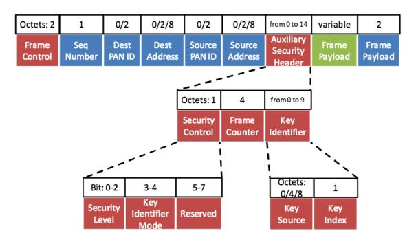
Fig. 2. The Auxiliary Security Header Structure
