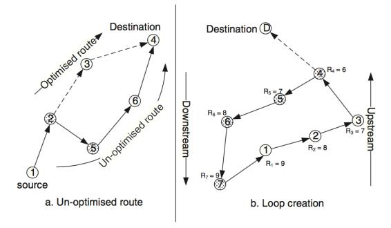
Figure 4. Unoptimised route and loop creation in rank attack scenario.
