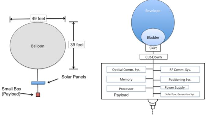
Figure 4. Project Loon Balloon and Payload Architectures
