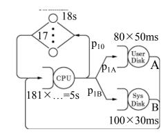
be: 8.88, 3.19, and 1.40 jobs at the CPU, disk A, and disk B, respectively. What were the response times of these devices?
