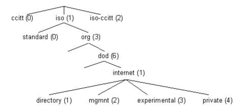
Figure 2 Partial depiction of the MIB naming hierarchy used by SNMP.
