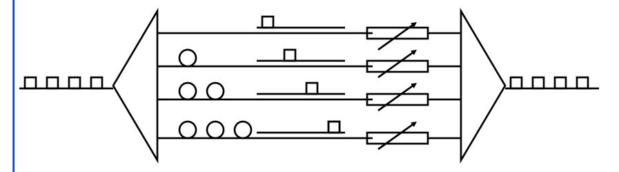
Splitter Delay lines Modulators Combiner
