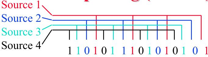
$\square$  Optics faster than electronics  $\Rightarrow$  Bit multiplexing.
