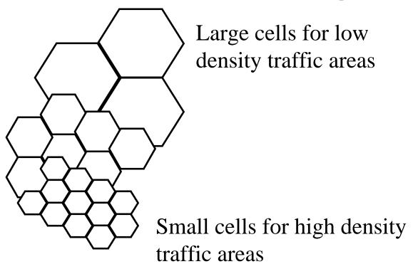
□ Cellular structure permits to reuse the frequencies and to distribute the resources depending on the traffic Arian Durresi
