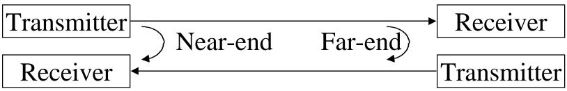
Echo Cancellation: Reflections from various distances along the path are estimated and subtracted from the received signal  $\Rightarrow$  144 kbps up to 4 km
