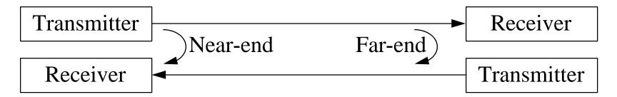
□ Echo Cancellation: Estimate echo and subtract from received signal. Transmitted signal is known. Reflections from various distances along the path are estimated and subtracted from the received signal ⇒ 144 kbps up to 4 km
