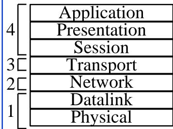
File transfer, Email, Remote Login ASCII Text, Sound Establish/manage connection End-to-end communication: TCP Routing, Addressing: IP Media Sharing: Ethernet How to transmit signal: Coding
