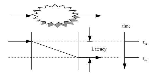
Figure A.1: Latency for a single bit
