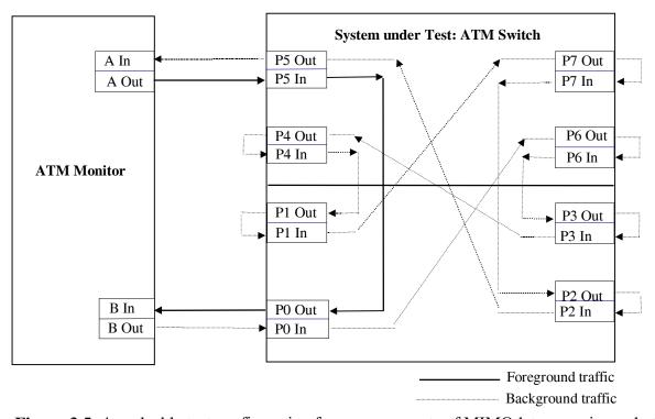
**Figure 3.5**: A scaleable test configuration for measurements of MIMO latency using only two generator analyzer pairs with 8-port switch and 7-to7 straight configuration for background traffic
