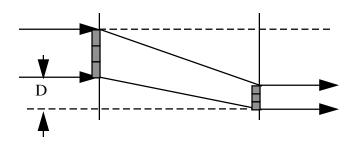
**Figure A.2bC**: Contiguous frames, Input rate < Output rate, Nonzero-delay switch In this case, the switch latency D is determined by a delay of the last bit. Here we have:
