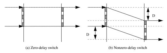
**Figure A.1aD**: Discontiguous frames, Input rate = Output rate, No change in gaps
