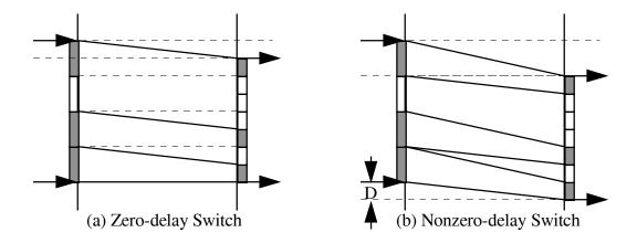
Figure A.2bD: Discontiguous frames, Input rate < Output rate, Expansion of gaps In this case, the switch latency D is determined by a delay of the last bit. Here we have:
