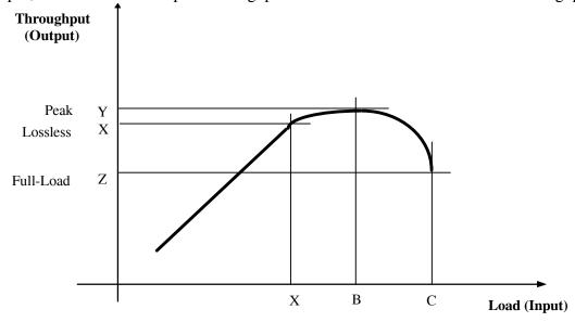
Figure 3.1: Peak, loss-less and full-load throughput
