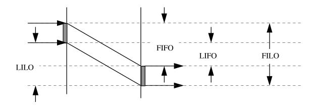
**Figure A.2**: Latency for multi-bit frames, input rate = output rate
