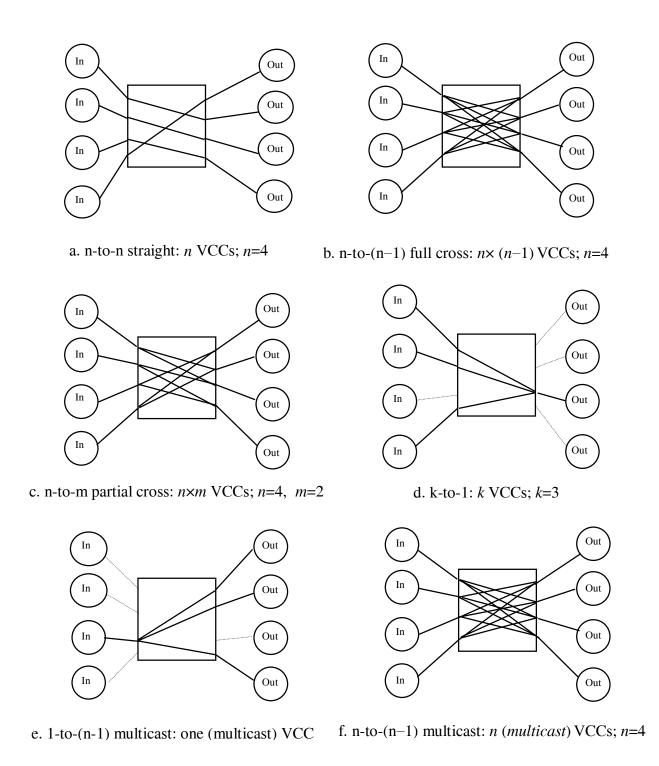
Figure 3.2: Connection configurations for foreground traffic
