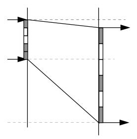
**Figure A.3bD**: Discontiguous frames, Input rate > Output rate, Expansion of gaps In this case, the switch latency D is given by:
