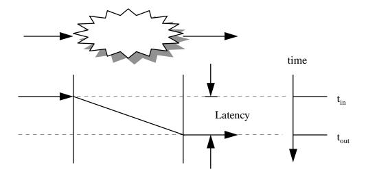
**Figure A.1**: Latency for a single bit
