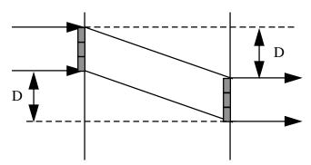
**Figure A.1bC**: Contiguous frames, Input rate = Output rate, Nonzero-delay switch In this case, the switch latency D is determined by a delay of the first bit (or the last bit). Here we have:
