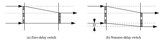
**Figure A.1cD**: Discontiguous frames, Input rate = Output rate, Compression of gaps In this case, the switch latency D is given by:
