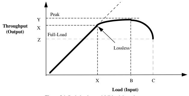
Figure 3.1: Peak, lossless and full-load throughput
