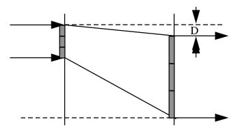
**Figure A.3bC**: Contiguous frames, Input rate > Output rate, nonzero-delay switch In this case, the switch latency D is determined by a delay of the first bit. Here we have:
