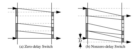
Figure A.2bD: Discontiguous frames, Input rate < Output rate, Expansion of gaps In this case, the switch latency D is determined by a delay of the last bit. Here we have:
