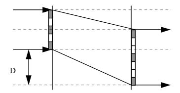
**Figure A.1bD**: Discontiguous frames, Input rate = Output rate, Expansion of gaps In this case, the switch latency D is given by:
