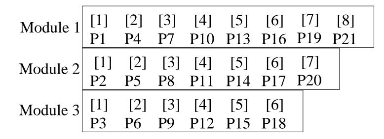
[x] indicates Port number in the module. Px indicates Port number used in our algorithm
