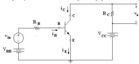
1. Draw the load line on the 2N2222A transistor characteristics shown on the reverse side and select a midrange operating point voltage ( $V_{CEQ} = V_{CC}/2$ ) that will allow essentially equal positive and negative voltage swings. Identify the corresponding operating point (Q point) currents.
