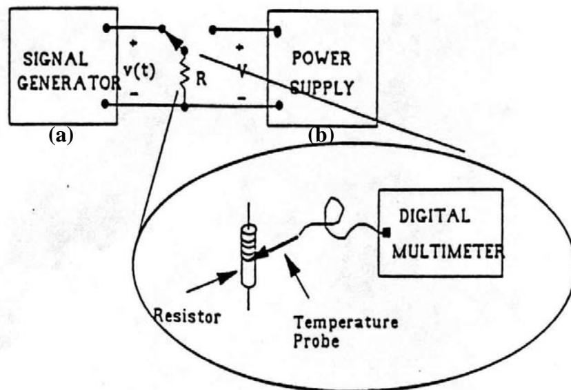
Figure 4.3: Setup for Resistor Power Measurement
