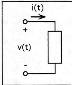
Figure 4.1: A two-terminal electrical element
