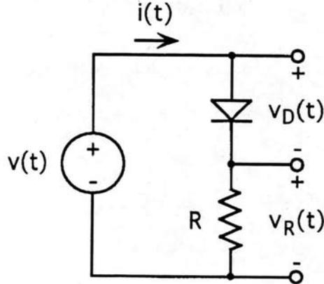
Figure 4.6: Diode Circuit
