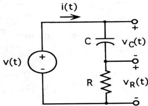
Figure 4.4: Series RC Circuit
