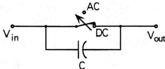
Figure 4.2: The circuit used to perform DC and AC coupling in the oscilloscope and in the DMM.
