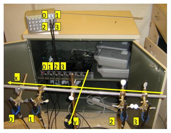
Connect the cables as shown above. This will put Microphone0 on the  $0^{th}$  element of the waveform array returned by the DaqAssistant. The angles Theta1 and Theta2 are shown below. The figure is oriented to match the photograph above.
