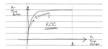
7. To determine the threshold, you need to look at the Receiver Operating Characteristic for the 2 distributions.
