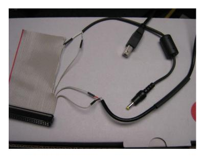
Cut of the ends of the USB cables and solder as shown. Plug ribbon cable into P5 – Pin 1 is toward center of sbRIO.
