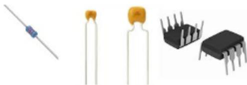
Each through-hole component has at least two legs that fit through holes in the PCB.
