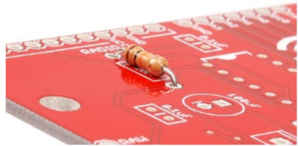
After soldering a component, it should lay flat on the PCB.
