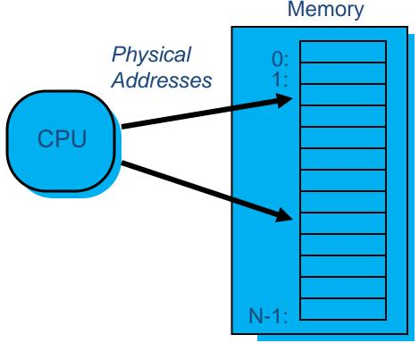
Addresses generated by the CPU correspond directly to bytes in physical memory
