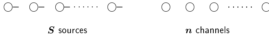
Figure 8.1: A full accessible loss system with S sources, which generate traffic to n channels. The system is shown by a so-called chicko-gram. The beak of a source symbolise a selector which points upon the channels (servers) among which the source may choose.
