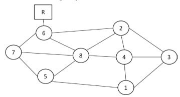
(3 points) Indicate on the diagram below, the structure of the spanning tree for this network, and <u>label all switch ports</u> as either root port (RP), designated port (DP), or blocking (B).
