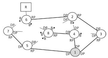
(2 point) Assume that the local area network has been assigned subnet 1.2.3.0/24. Consider host 1.2.3.4 attached to bridge 7 that wants to send a packet to host 1.2.4.5. How would host 1.2.3.4 obtain the MAC address needed to reach host 1.2.4.5 and what path would packets destined for host 1.2.4.5 follow in the switched network?
