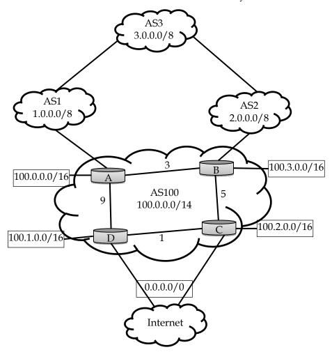
a) Specify the routing table at router A, and for each entry identify the next hop(s) in the form of either a local connection, or connections to internal routers, or a neighboring AS.
