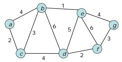
a) Are any network links never used when sending packets **to** a host Z connected to router *g*? Simply mark these links with an **X** on the diagram, but explain your reasoning. Assume that the topology is stable, that the link costs do not change and that *g* advertises a route to Z.
