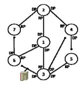
(i) Under the spanning tree configuration shown in the figure, is any bridge not forwarding data packets? If no, identify for each bridge the LAN segments to and from which it forwards data packets. If yes, explain why some bridges may not be forwarding data packets.
