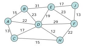
b) Suppose that router *C* is the PIM DR for some layer 2 subnet, and that a host *X* in that subnet sends an IGMP report for address 229.1.2.3. Assume that *J* is the RP for 229.1.2.3 and that no other routers are currently participating in 229.1.2.3. What does router *C* do at this point? Which routers eventually add forwarding state for 229.1.2.3 as a result of *C*'s action?
