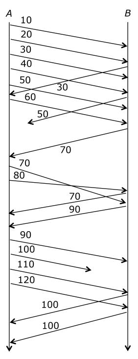
7. (10 points) The diagram at right shows two TCP senders at left and the corresponding receivers at right. Both senders use TCP *Tahoe*. Assume that the MSS is 1 KB, that the one-way propagation delay for both connections is 100 ms and that the link joining the two routers has a bandwidth of 16 Mb/s. Let *cwnd*<sub>1</sub> and *cwnd*<sub>2</sub> be the values of the
