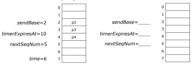
Suppose that at time 7, the application passes us a new payload to be sent and at time 12, we receive an ack with sequence number 3.
