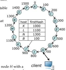
Suppose the client shown in the diagram sends a get request to node *H* with a *Client* key string of "flapjack", and that *hash*("flapjack")=513. List the servers through which this request would pass, assuming that the key string does not appear in any node's cache.
