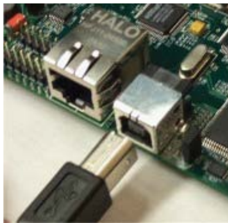
Figure 4-4: Connect the USB Type B Connector to the Starter Kit Board Connector
