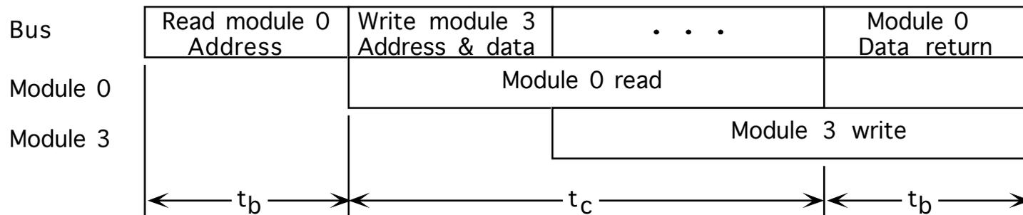
With interleaving of  $2^k$  modules, and  $t_b < t_c/2^k$ , it is possible to get a  $2^k$ -fold increase in memory bandwidth, provided memory requests are pipelined.
