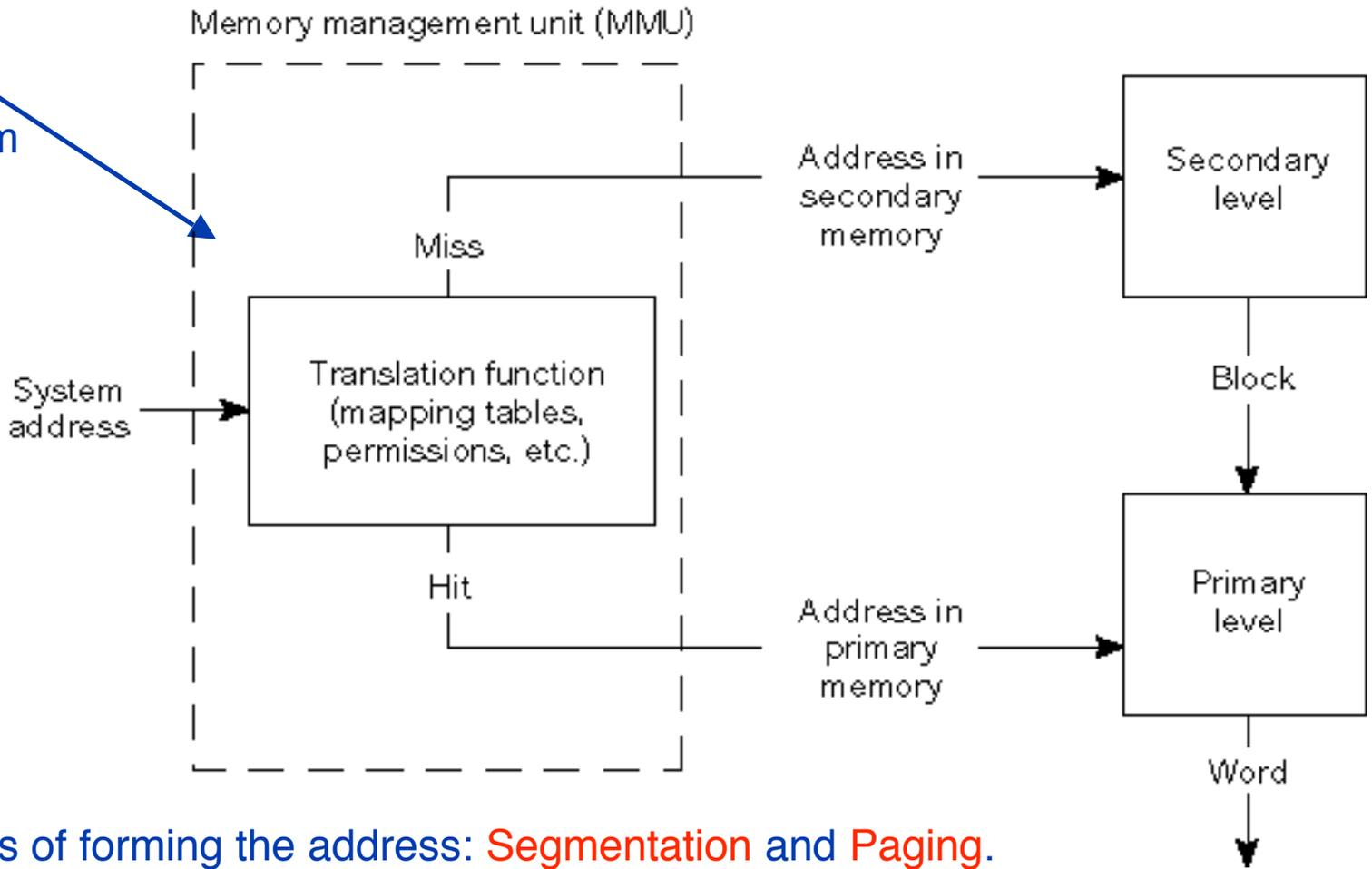
Two ways of forming the address: **Segmentation** and **Paging**. Paging is more common. Sometimes the two are used together, one “on top of” the other. More about **address translation** and **paging** later...
