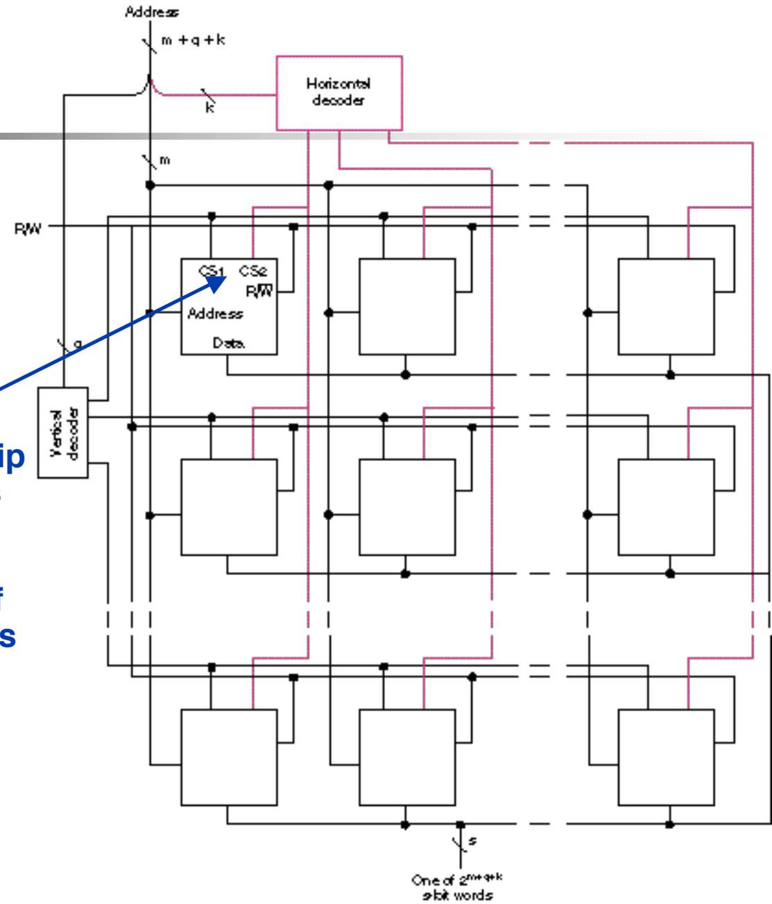
Multiple chip select lines are used to replace the last level of gates in this matrix decoder scheme.
