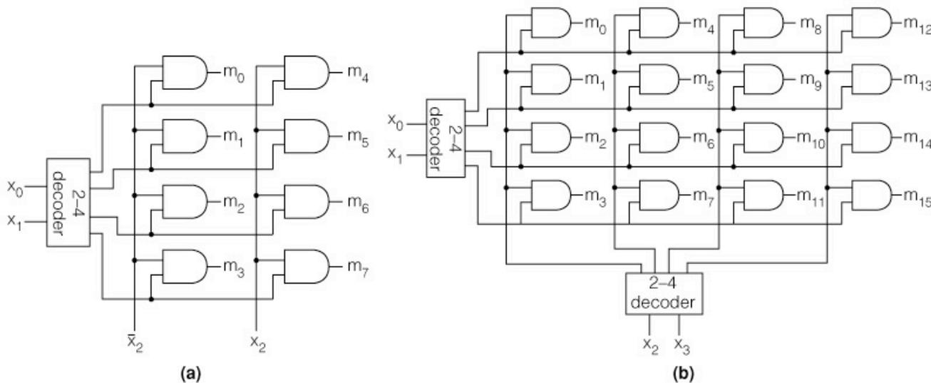
3-to-8 line tree decoder constructed from 2-input gates.
