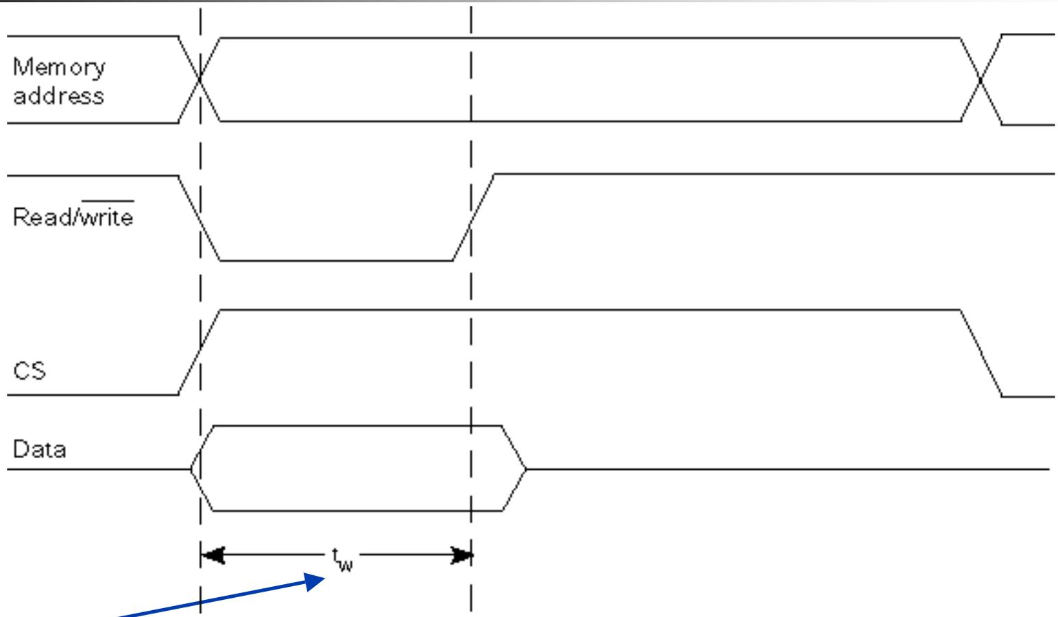
**Write time**—the time the data must be held valid in order to decode address and store value in memory cells.
