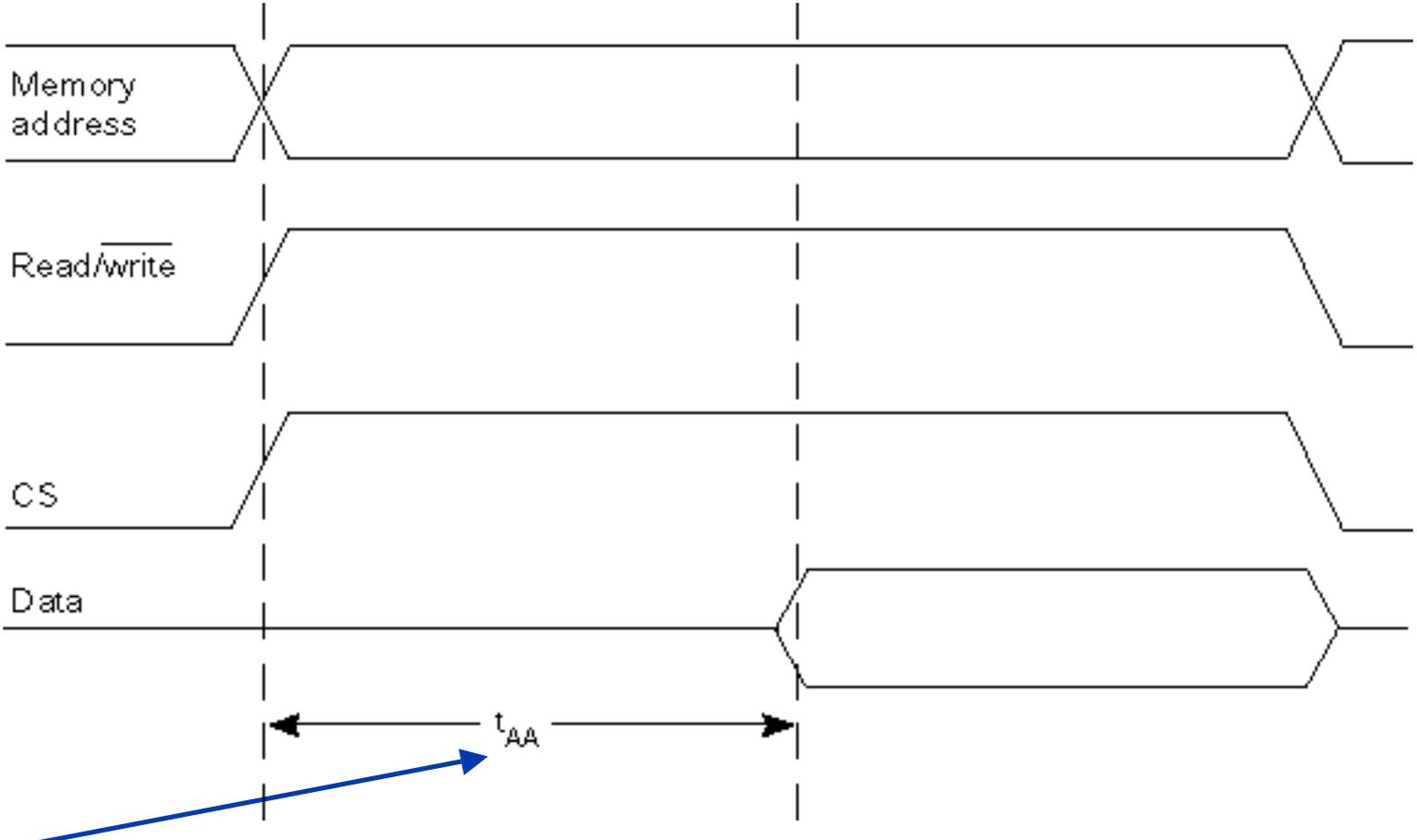
**Access time from Address**— the time required of the RAM array to decode the address and provide value to the data bus.
