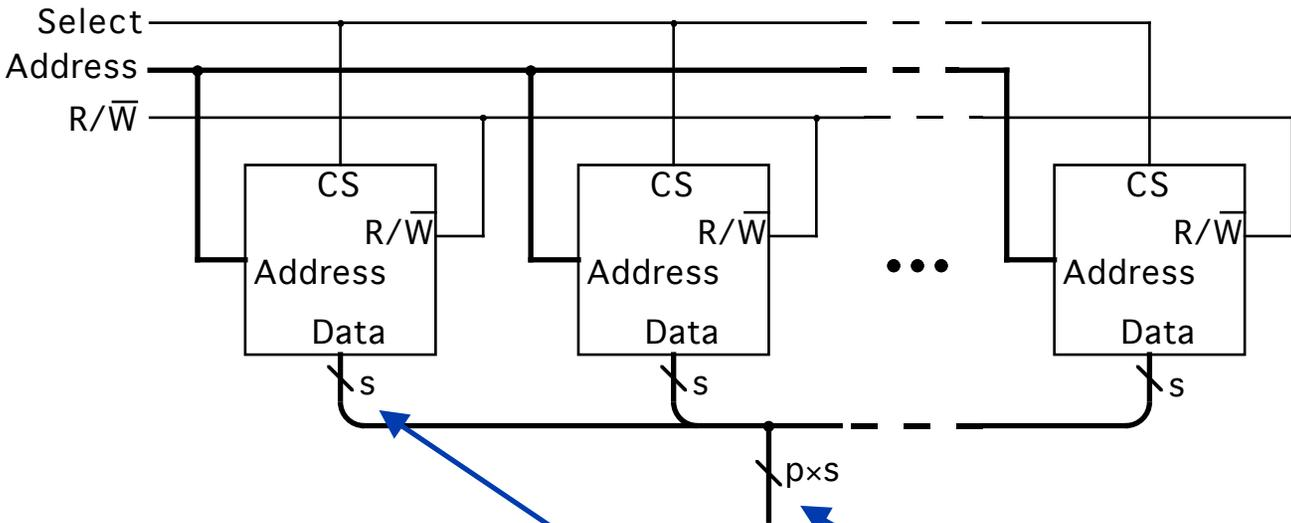
P chips expand word size from s bits to p x s bits.
