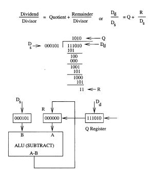
Division Procedure: If (A-B) > 0, load (A-B) into R and prepare a '1' for the Q register.
