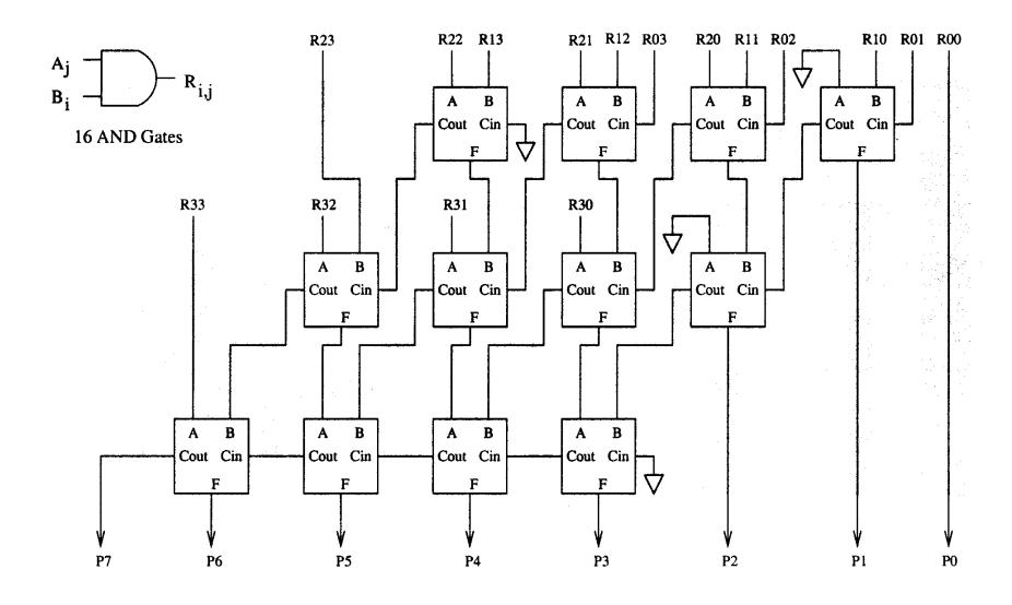
This approach allows the time delay of each (intermediate) stage to reduce to 2 gate delays!
