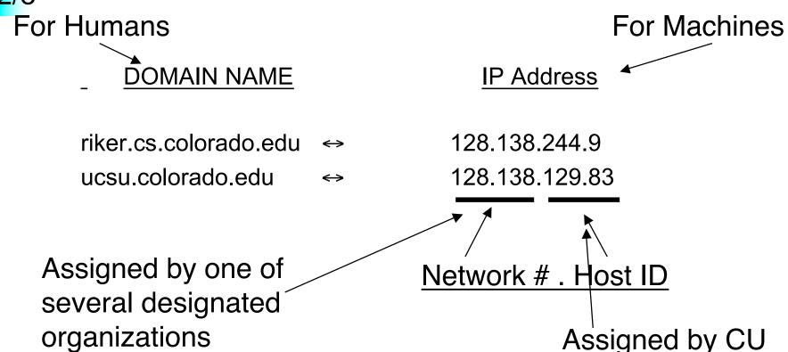
Originating machine requests lookup of IP address from a Domain Name Server, using Domain Name Service
