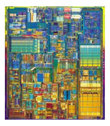
Intel Pentium 4 0.13µ process 55 million transistors 2.4GHz clock 145mm<sup>2</sup>
