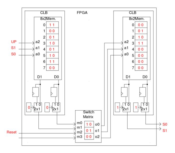
1. Design a 2 bit up/down counter with reset using the FPGA circuit below.
