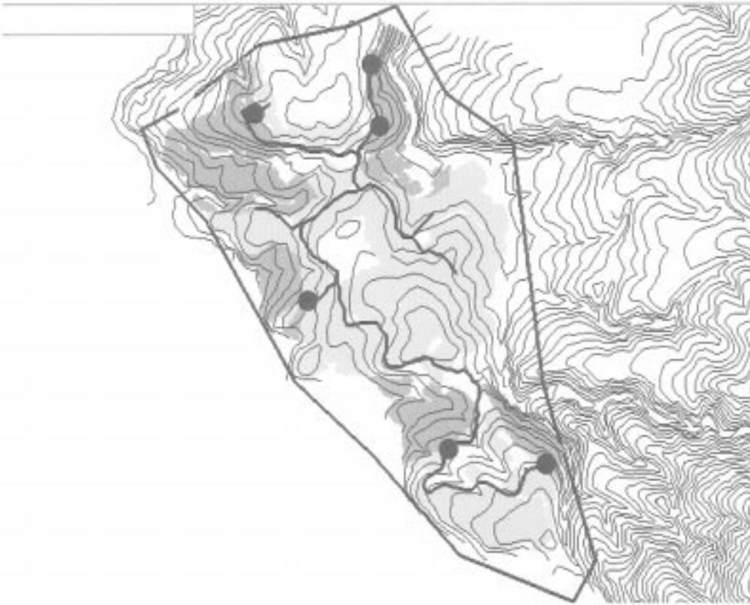
Figure 6: In this PLANEX output example, the light shaded area shows the area harvested with skidders, while the dark shaded area represents tower harvesting. The full lines show the connecting road network, while the black dots indicate the position of the towers.
