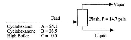
Design Specification: Mole fraction of C in vapor = 1%.
