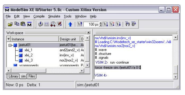
You can either use the dialog boxes to enter commands or type them in on the command window. You can also write a script file of ModelSim commands. Change signals b and c to 0. Now run the simulation by typing "run" on the command window.
