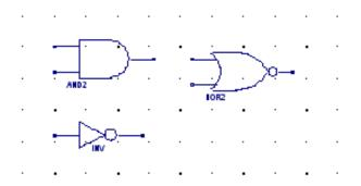
Arrange the three symbols so they are approximately located on the schematic like shown above. It is recommended that you zoom in so the inputs and outputs of the symbols can easily be seen. Next, the schematic will be wired by using the Add Wire tool.
