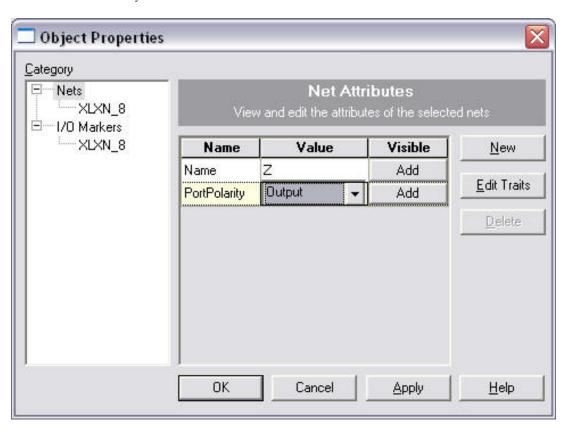
Change the Name Value to Z and the PortPolarity Value to Output. Click OK. Repeat this process for the three inputs (A, B, C). Be sure the PortPolarity is set to Input.
