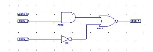
Next, double left-click on the I/O marker for the output of the circuit (the NOR2 output).
