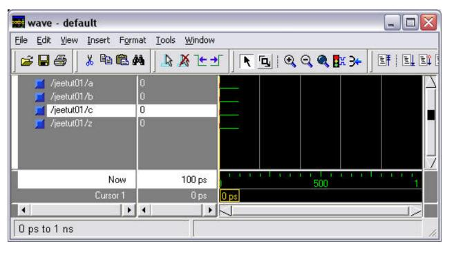
Next force inputs a, b, and c to 1, 0, 0 respectively. Type in run again. Repeat until you've covered all input states. Does the output waveform agree with the boolean expression for this circuit?
